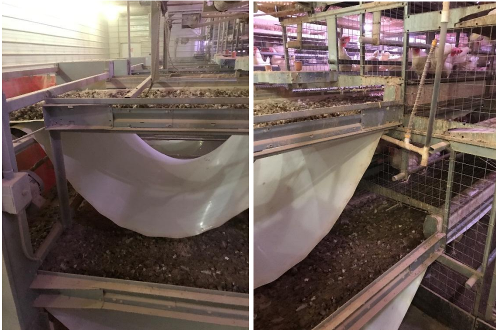
Figure 2. Layer house manure belt system (photo credit: Chai).
