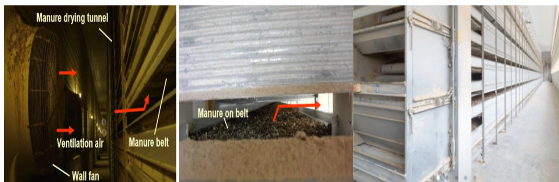
Figure 3. Manure drying tunnel on a layer farm. (photo credit: Ni et al., 2010; Chai et al., 2012; Big Dutchman).
