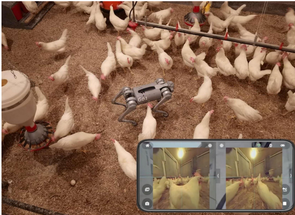
Figure 4. Robotic machine vision method for tracking dead chickens and floor eggs.
