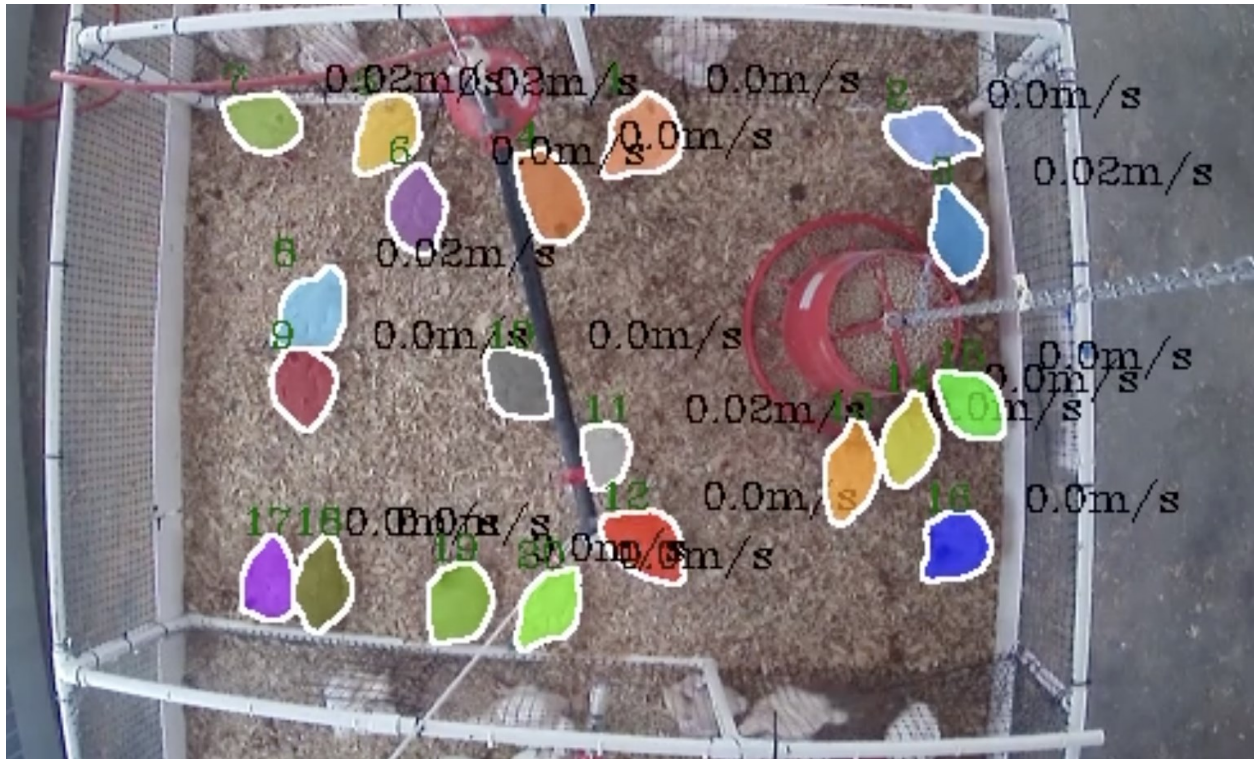
Figure 3. Track and detection speed of broilers (The green number indicates the tracking number, while the black number represents speed).
