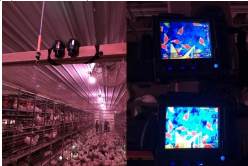
Figure 2. Thermal cameras setup at 6.6 ft above litter floor in the cage-free house.
