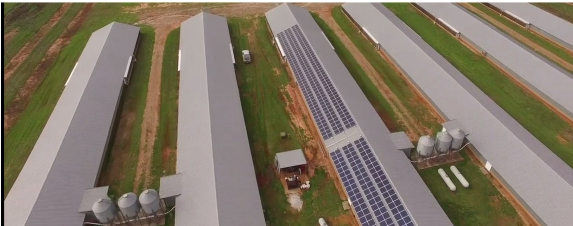
Figure 4. A poultry house-roof mounted solar power systems (photo credit: Coastal Solar Solutions).
