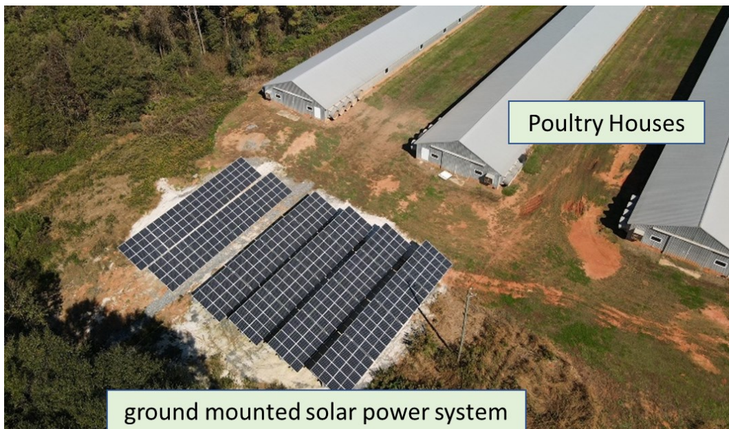
Figure 1. A ground mounted solar power system with panels on concrete floor (photo credit: Lilong Chai).
