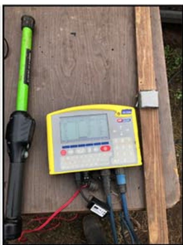
Figure 2 – Data Measurement Devices: Allflex EID Reader, Tru-Test Indicator and tape measure
